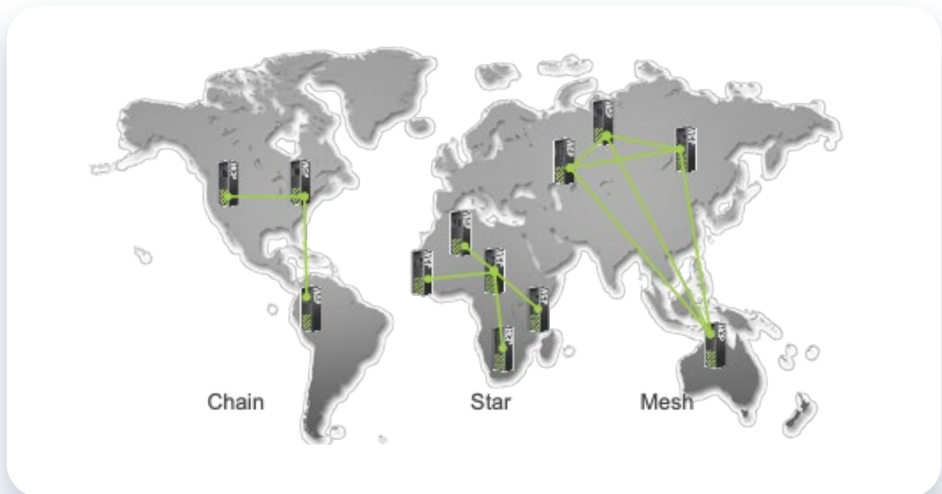
Figure 14. Chain, Star and Mesh Configurations
